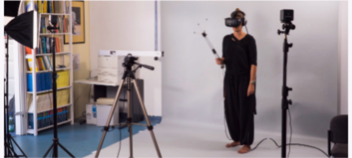
Fig. 5. A user interacting with Shifty in our experimental setup. The user wears the HTC Vive and headphones. The rigid-body target on the proxy is tracked by an OptiTrack system.
